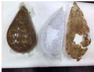
Figure 1: A kenaf helmet shell with fibre strips (left) and kenaf helmet shell (right).
